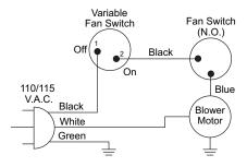
Figure 30 - Blower Wiring Diagram for Thermostat-Controlled Models
